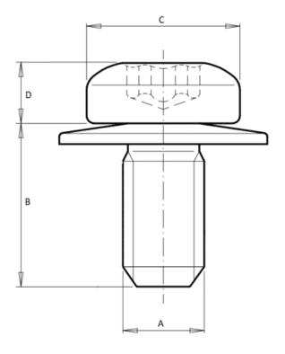
Categories: Applications Screws, M6 with washer, Metric special screws M6, Our Products
